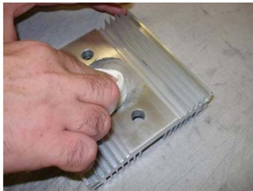
The heatsink mounting surface should appear lightly abraded as shown.
