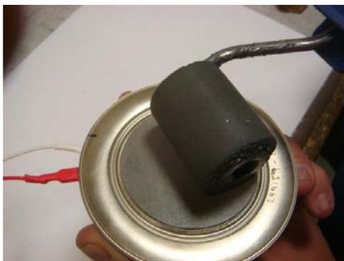
The contact surface should have a thin film of grease applied to the surface as shown.
