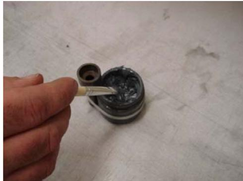
Apply the grease to the heatsink close to the spiro pin as shown.
