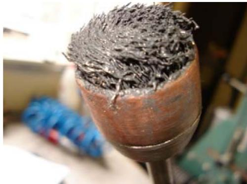
Leave the heatsink slurred with the thermal grease until the device is ready to be mounted.
