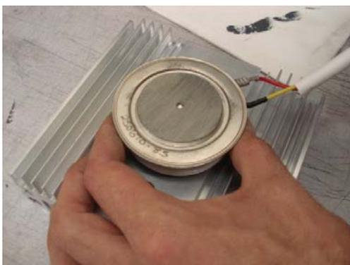
Note that a small amount of grease should be squeezed out of the device/ heatsink joint when the clamp is tightened. Excessive grease will cause a high volt drop across the joint and affect heat transfer. The bead of grease should be no more than 0.1mm.
