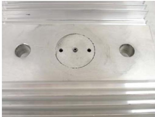
Close up of the device mounting area after the device was removed.
