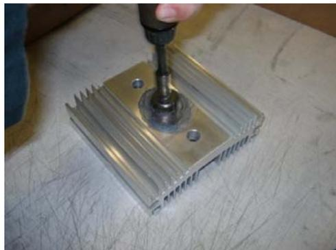
Note that the rotary wire brush must be replaced when the bristles are too short.
