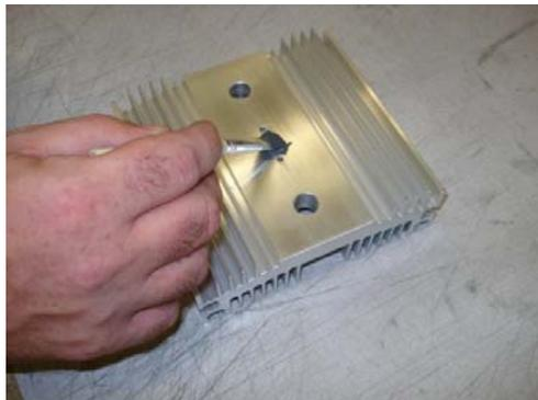
An air operated rotary wire brush is used to abrade the paste onto the heatsink.
