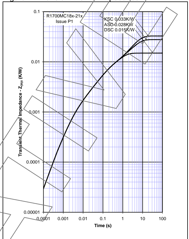
Figure 2 - Transient thermal impedance
